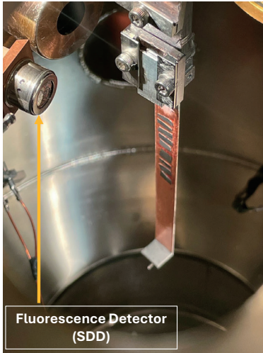
(a) Experimental setup for IPFY mode@TLS 20A beamline
